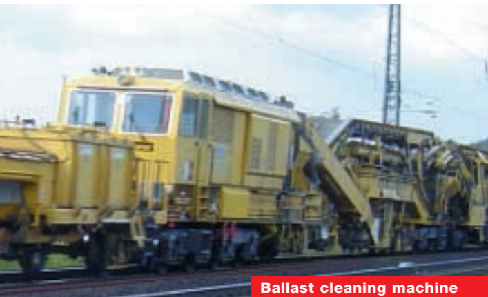
Ballast cleaning machine
